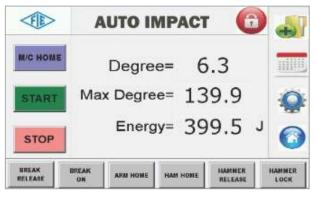
In Auto Impact-30, Pendulum will lift, specimen will get loaded and pendulum will release automatically. Once specimen breaks, result will display on digital panel, and auto brakes will apply immediately.
